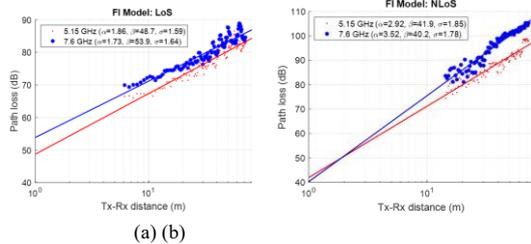
Figure 2: Path loss model fitting of outdoor measurement results
