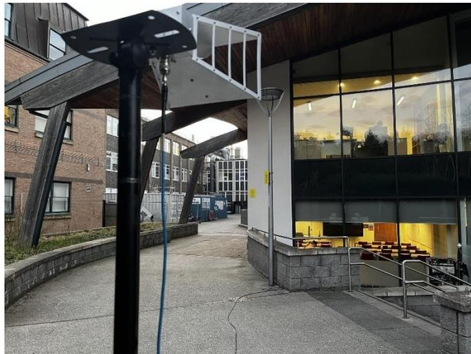
Figure 5 Scenario of measured modern building entry loss
