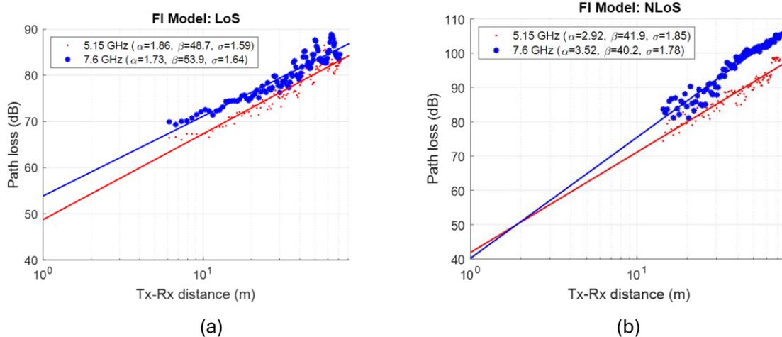
Figure 4. Path loss at 5.15 GHz and 7.6 GHz, for (a) LoS, (b) NLoS
