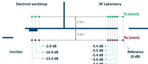
Figure 3: Measurement setup and results of penetration loss
