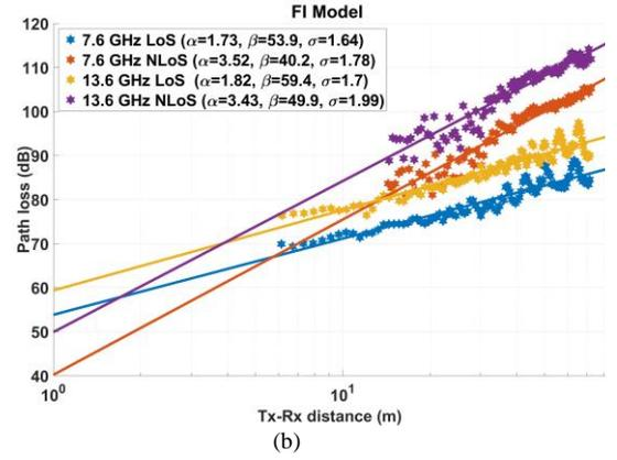
Fig. 6. Fitting results of path loss (a) CI model, (b) FI model.
