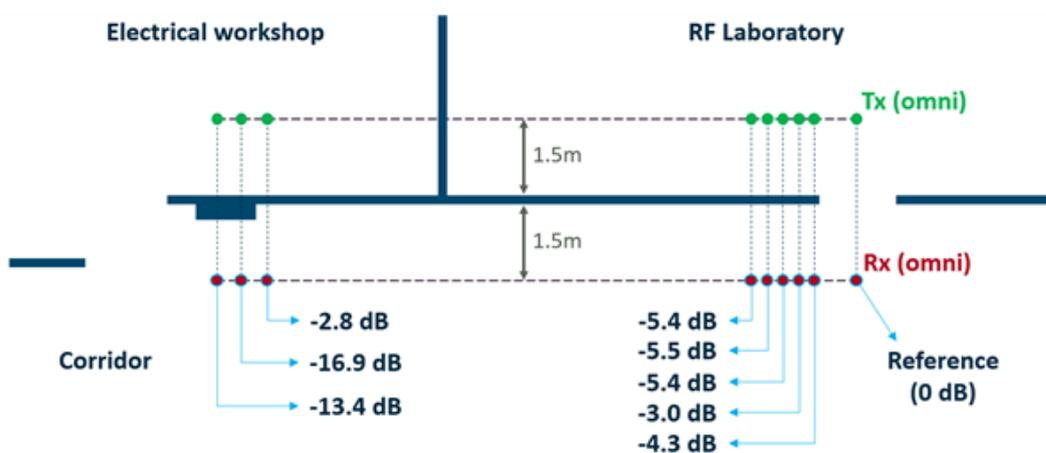
Figure 4. Penetration loss through indoor wall
