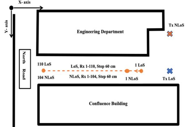
Fig. 2. Layout of the outdoor measurement scenario.
