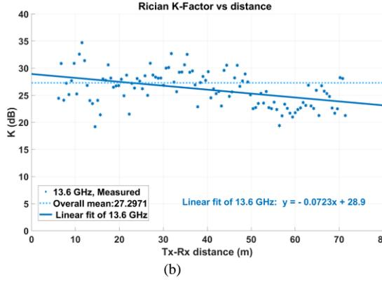
Fig. 5. Rician K-Factor vs distance for (a) 7.6 GHz and (b) 13.6 GHz
