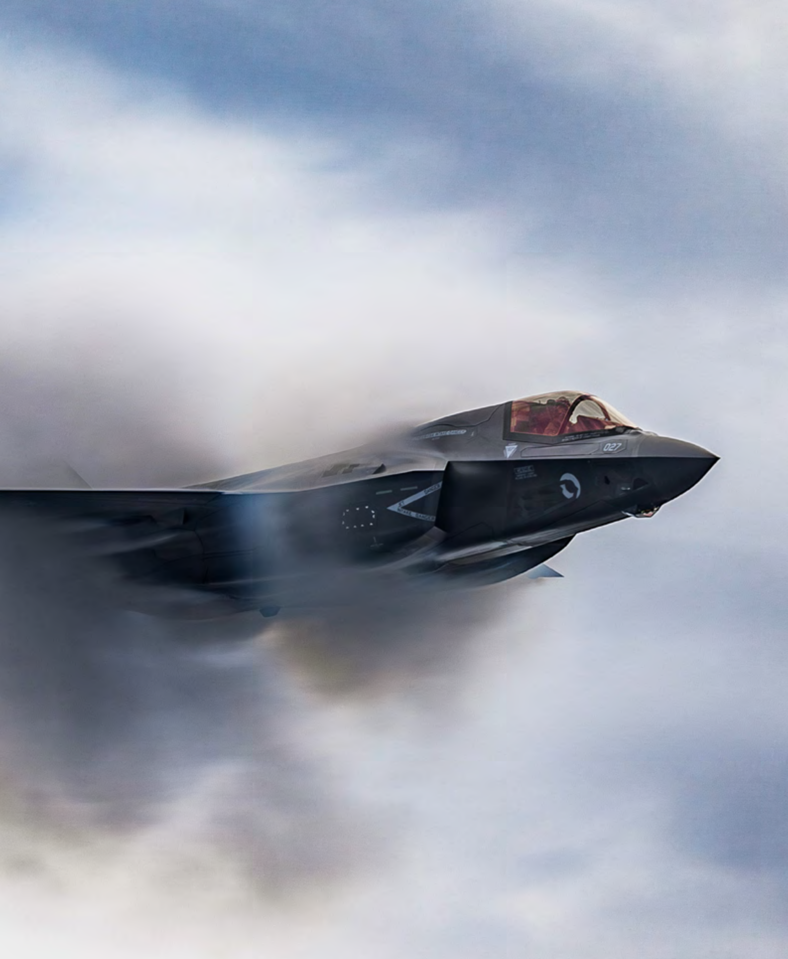
An F-35B Lightning Jet creates a vapor cone as it flies past the Aircraft Carrier during flight deck operations in July 2023. Credit: AS1 Natalie Adams
