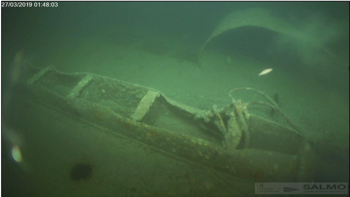
PRINCE OF WALES – Bottom of the hull showing section of plate peeled back by salvors.
