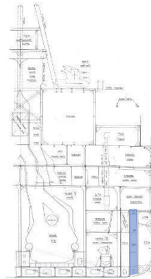
Arrangement of bottom/side fuel tanks at Frame 156 (amidships)
