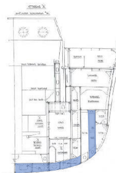
Arrangement of bottom/side fuel tanks at Frame 89 (forward)
