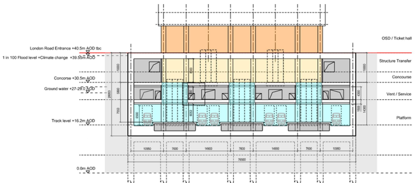
Figure 15 - Option B1 Cross Section
