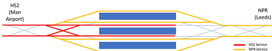
Figure 5 - Layout and station approach
