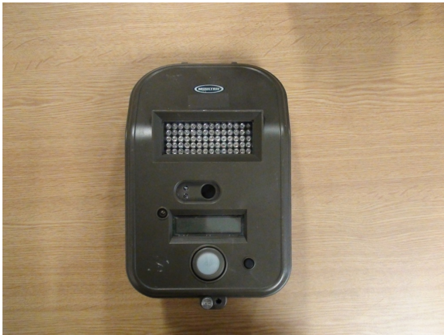
Figure 5.4. Trail camera used to measure activity
