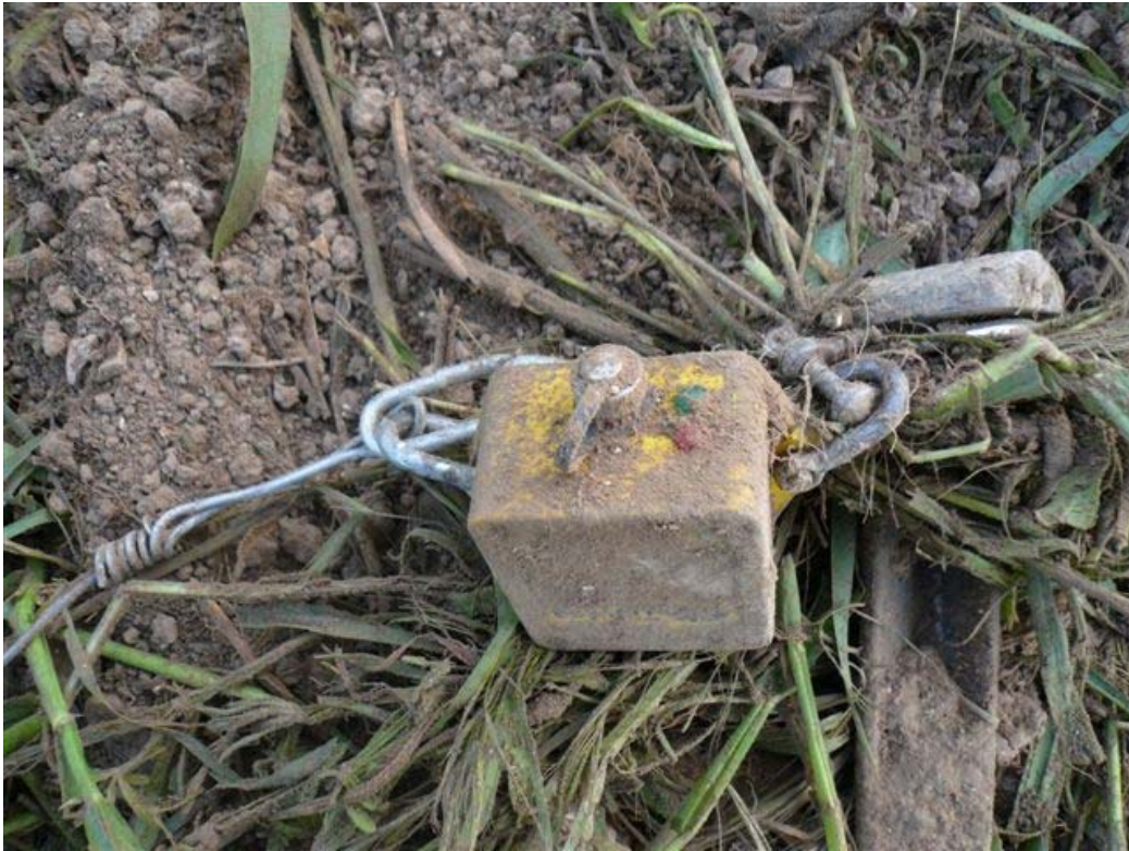
Figure 5.10. The anchor-swivel of the snare that broke following capture of a badger. The anchor-swivel was distorted and the snare cable could not be rotated at this swivel.
