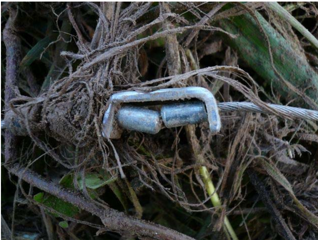
Figure 5.11. The middle swivel of the snare that broke following capture of a badger. The two ferrules within the swivel are jammed together and the snare cable did not rotate at this point.
