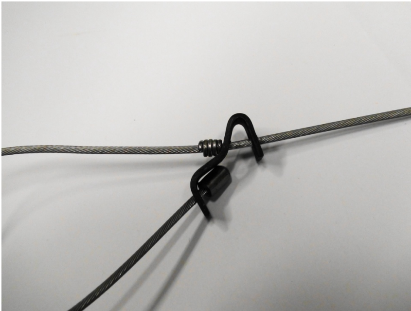
Figure 5.15. Illustration of non-running eye caused by the eye plate deforming during the 5kg test on snare B.
