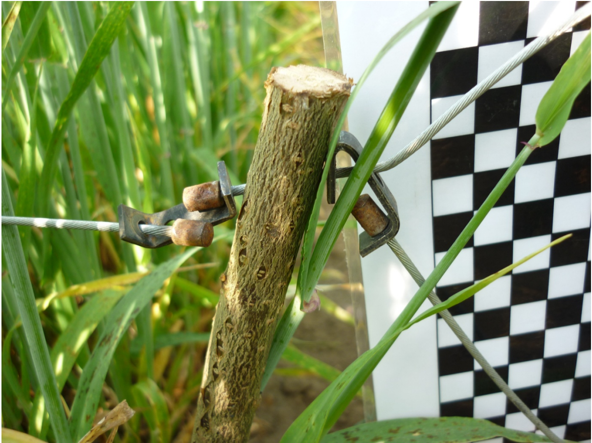
Figure 2.16. An example of the swivel, running eye and crimps typical of the majority of snares examined during the field visits. In this case, a wooden tealer has been used to support the snare. The checkerboard was used to measure dimensions without the need to handle the snare.
