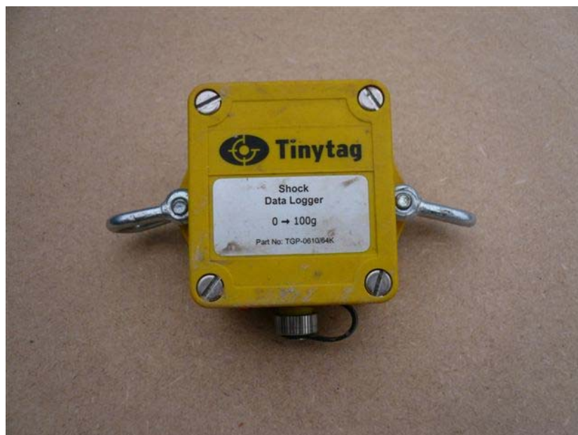
Figure 5.3. Tinytag data logger used to record activity during the trials.
