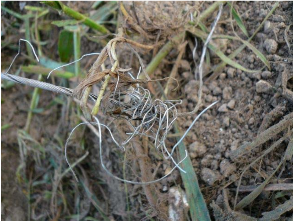
Figure 5.12. Fraying of the snare cable that broke following the capture of a badger
