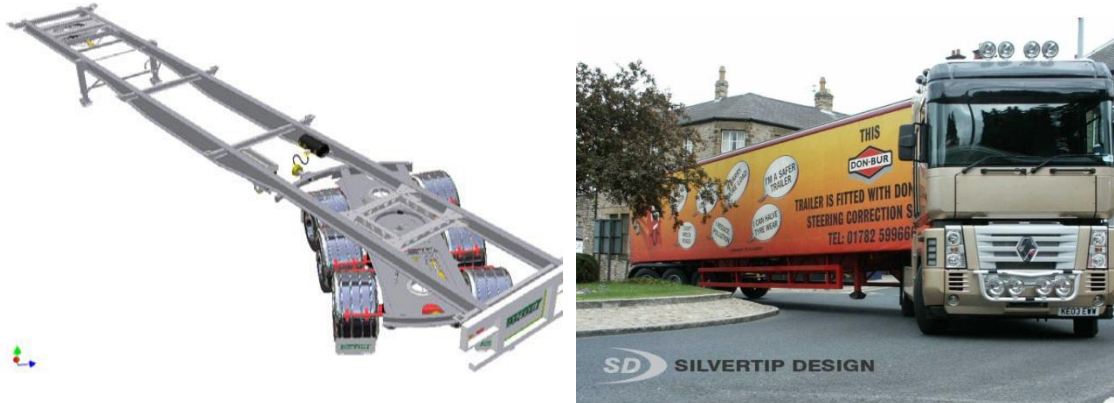
Figure 3. Examples of pivotal bogie systems from Trackaxle (left) 4 and Don-Bur/Silvertip design (right) 5 .
