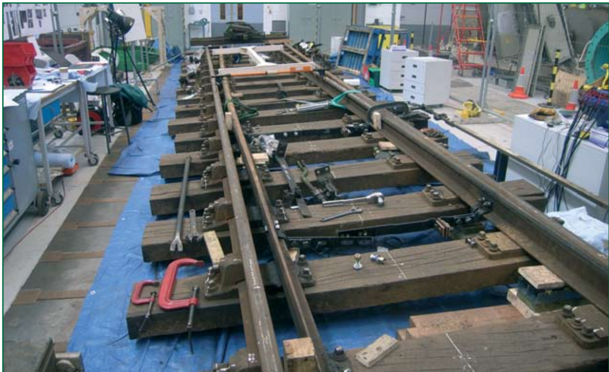
Figure 6: Points 2B switch section in laboratory
