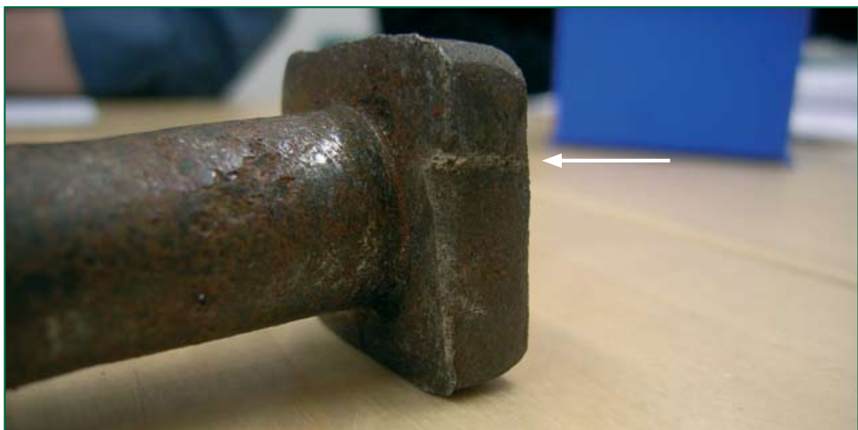
Figure 13: Indentation in lock stretcher bar bolt head
