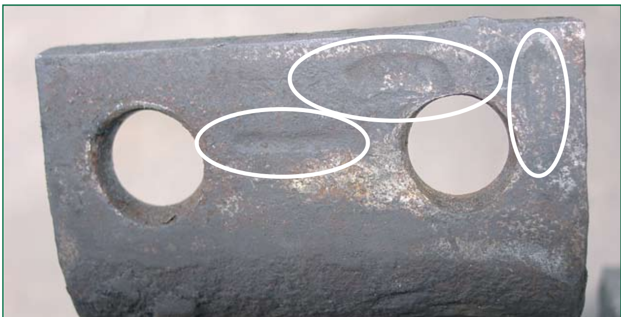
Figure 25: Indentations imprinted into the mating face
