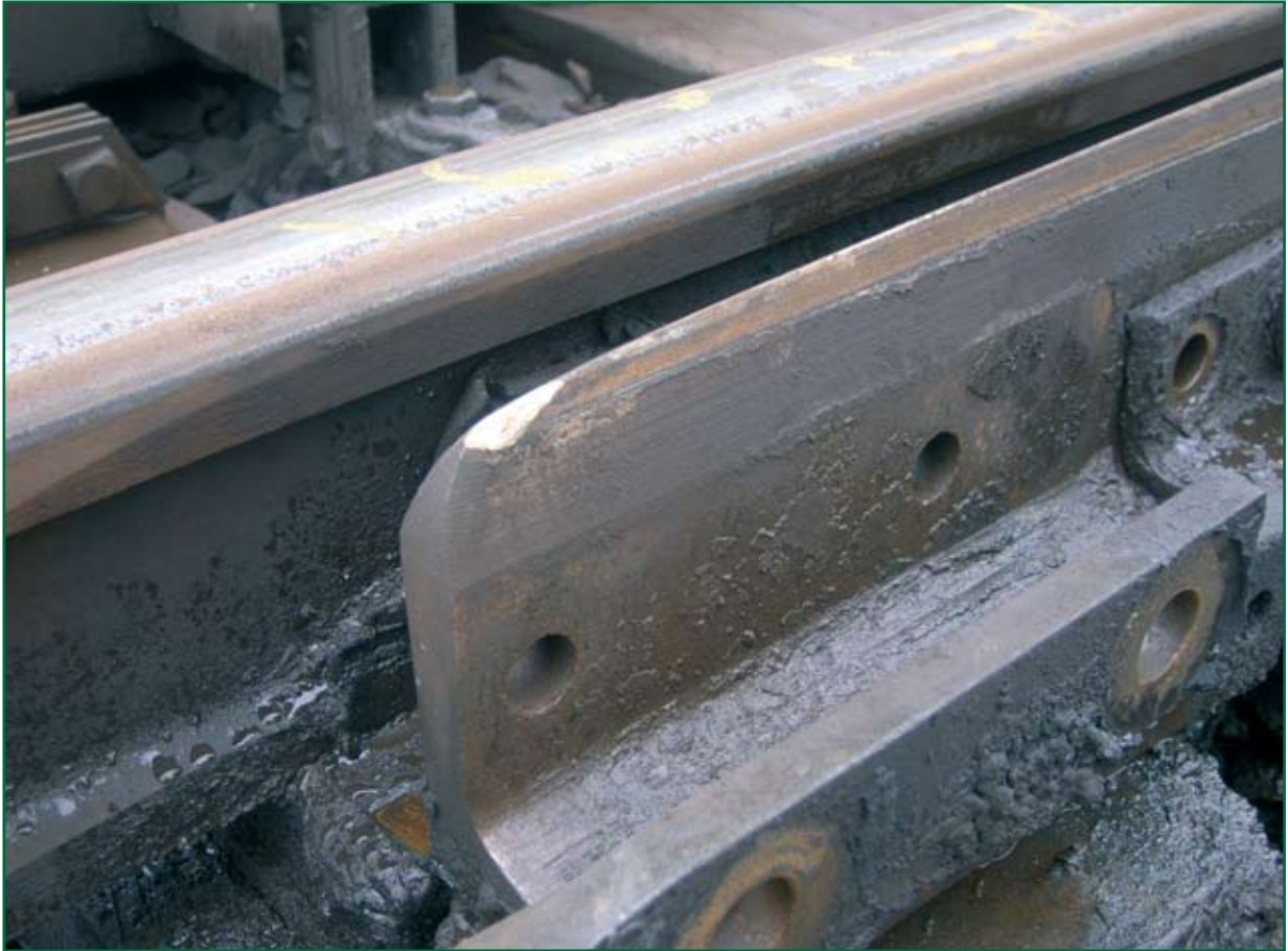
Figure 8: Bruise to the tip of the left-hand switch rail
