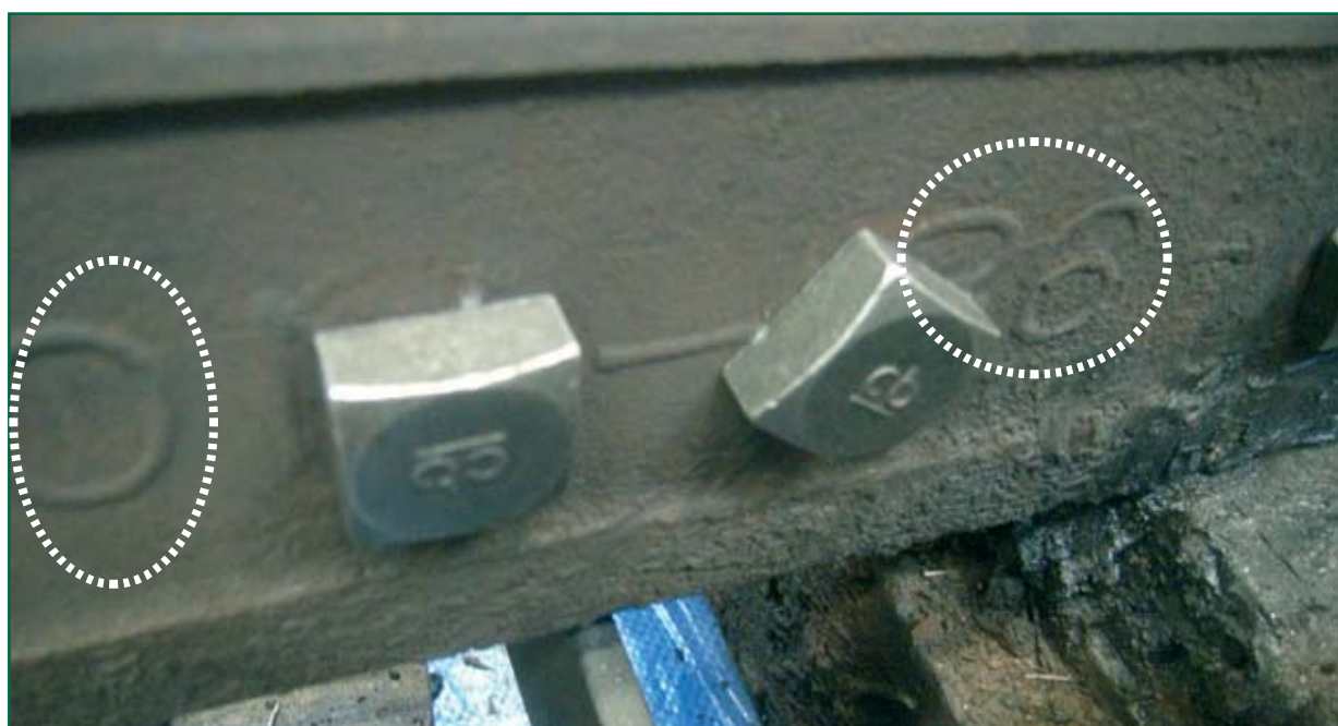
Figure 11: Rail branding on left-hand switch rail (Note: new bolts added for testing purposes)
