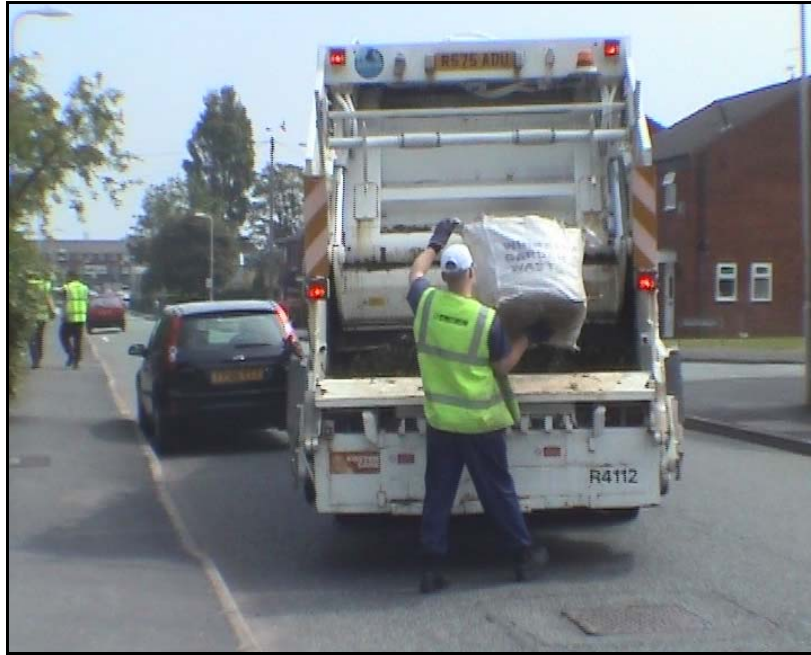
Figure B1 Emptying of reusable bag of green waste into back of an RCV
