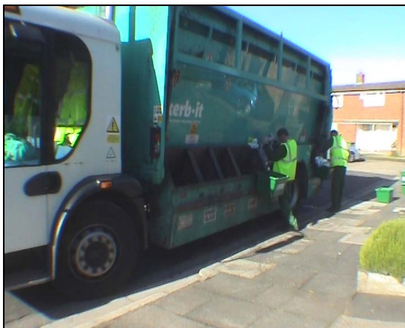
Figure B3 Kerbsider vehicle used in observed dry recyclable collection and sort system
