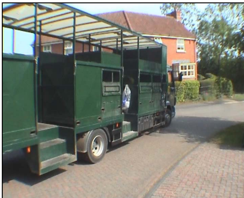
Figure B2 Stillage vehicle used in observed dry recyclable and food waste collection system
