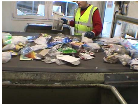
Figure F3 Hand sorting of dry recyclable material at an MRF
