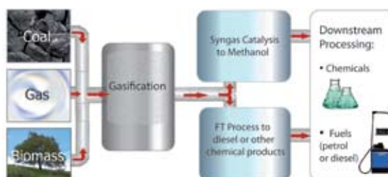
Diagram of gasification process
