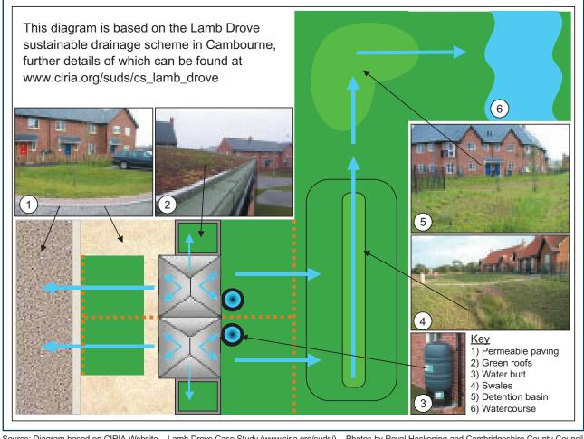
Figure 13 - Diagram of how SuDS can be used on a local scale
