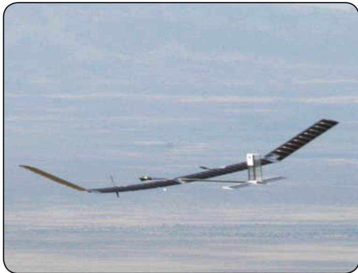
Zephyr is a High Altitude Long Endurance (HALE) UAV, which uses a combination of innovative light weight airframe material, solar cell and battery technologies to provide sustained performance at high altitude. (Image courtesy of QinetiQ®)
