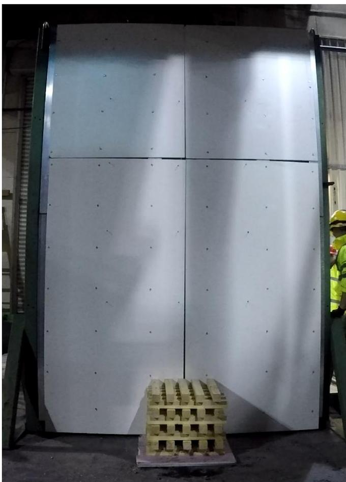
Figure G11 – Sample S25 HPL panels installed on the rig
