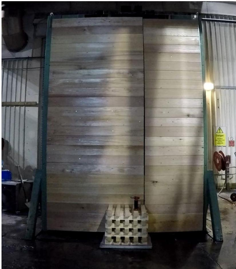
Figure G26 – Sample S28 timber cladding installed on the rig
