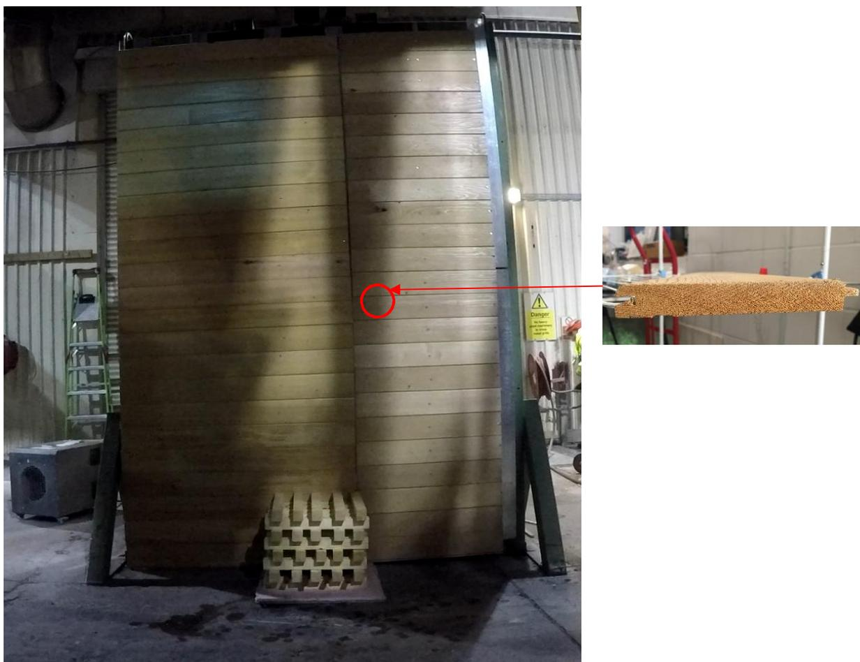
Figure G21 – Sample S27 timber cladding a) installed on the rig (left) and b) cross sectional profile of tongue and groove (right)
