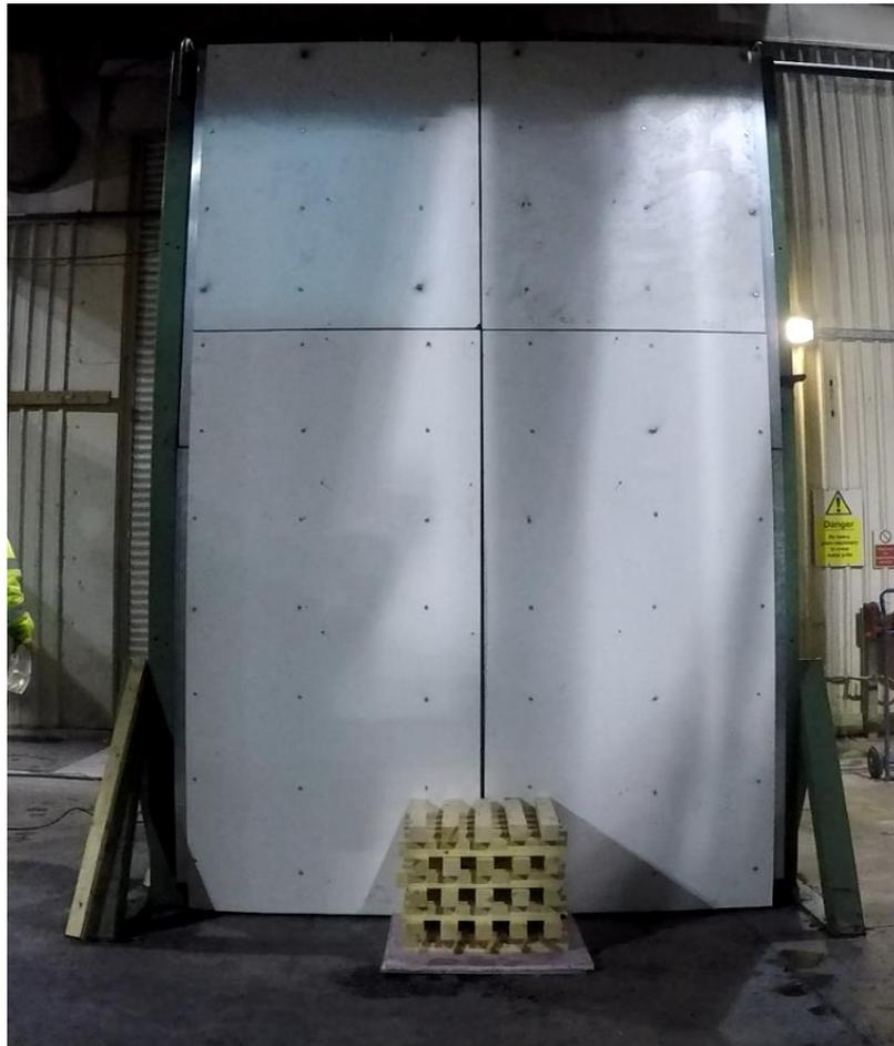
Figure G16 – Sample S26 HPL panels installed on the rig
