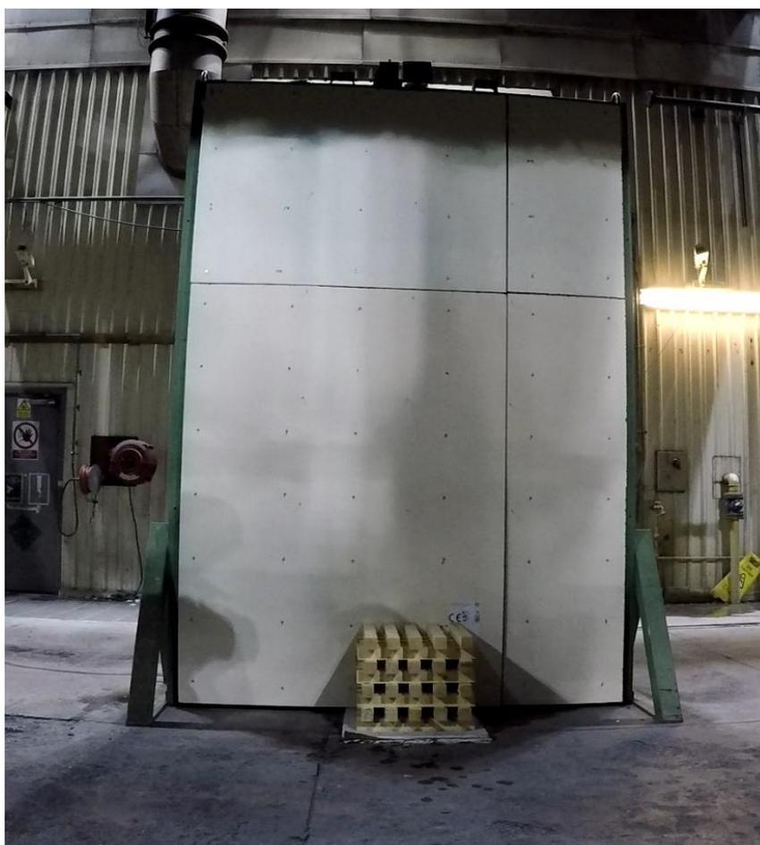
Figure G1 – Sample S23 HPL panels installed on the rig
