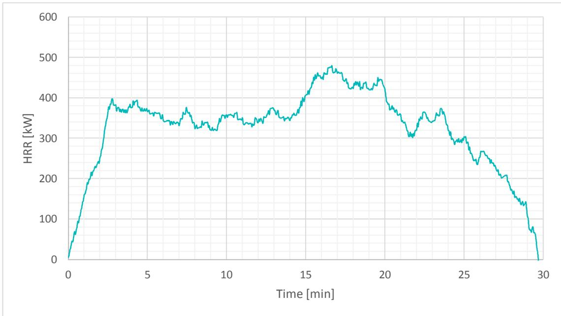
**Figure G23 – Heat release rate measured during the fire, including the source**
