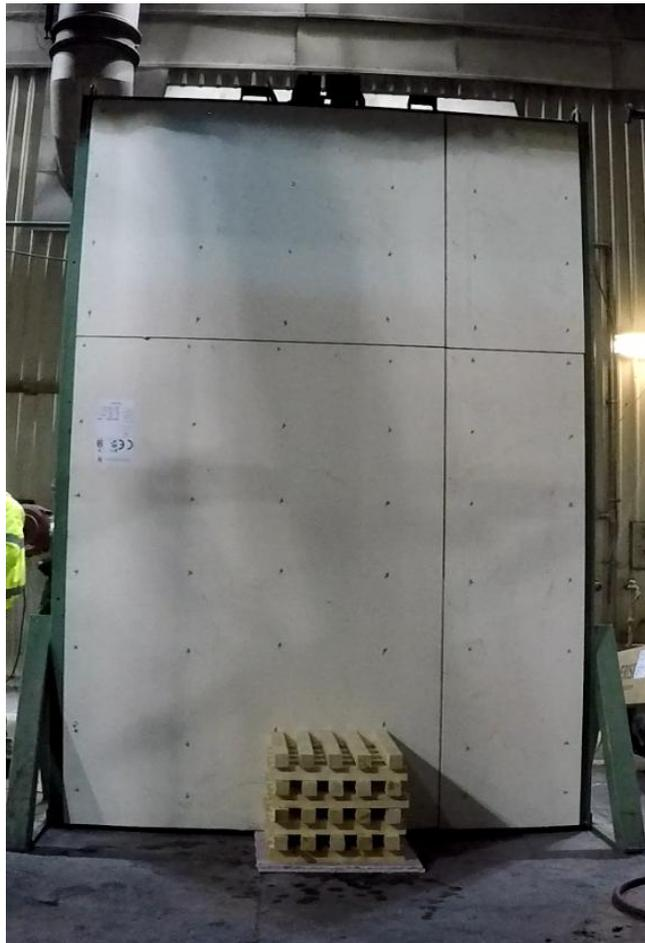
Figure G6 – Sample S24 HPL panels installed on the rig
