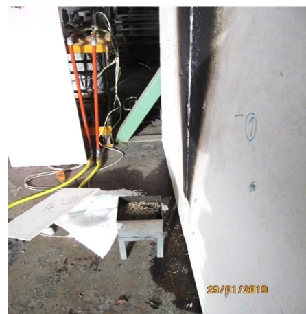
Figure D16 – Burner 100 mm from face of the calcium silicate board
