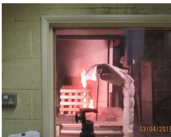
Figure D23 – Ignition of timber crib inside oxygen consumption calorimeter (Single Burning Item test apparatus [8] )
