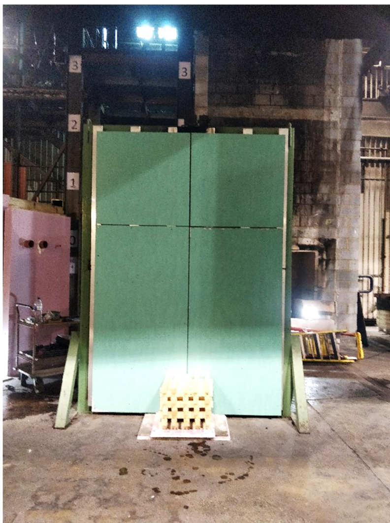
Figure D33 – ACM PE material installed on the experimental rig
