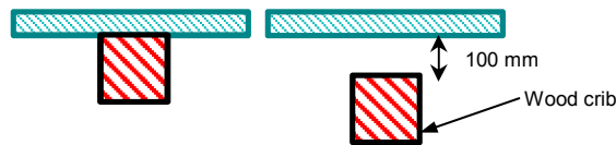
Figure D7 – Plan view sketch showing the wood crib arrangements in the model
