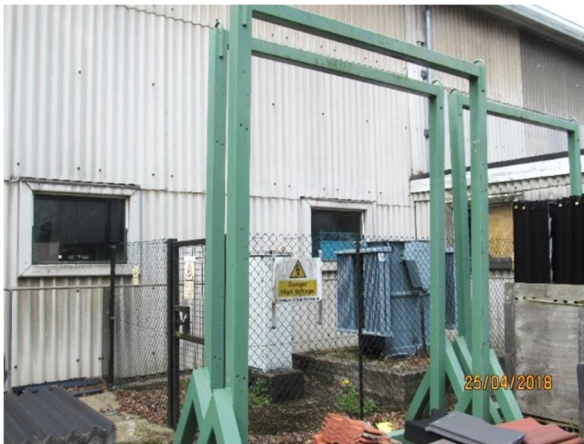
Figure D8 – Steel frame used to construct experimental rig
