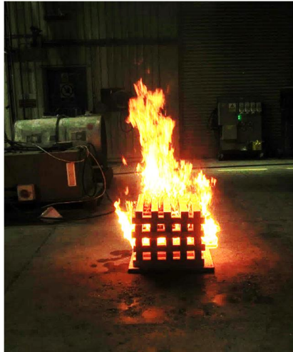
Figure D25 – Timber crib alight under 9 m by 9 m calorimeter hood (open calorimetry)
