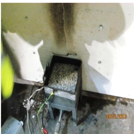
Figure D15 – Burner tight up against calcium silicate board
