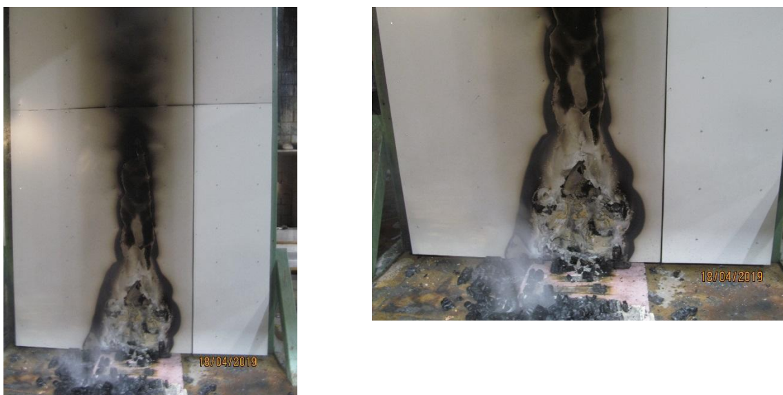
Figure D42 – Post fire observations
