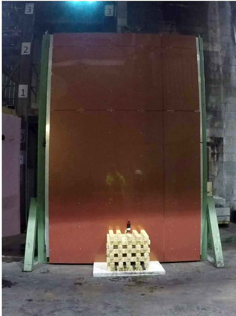
Figure D28 – ACM FR material installed on the experimental rig for ACM fire 1
