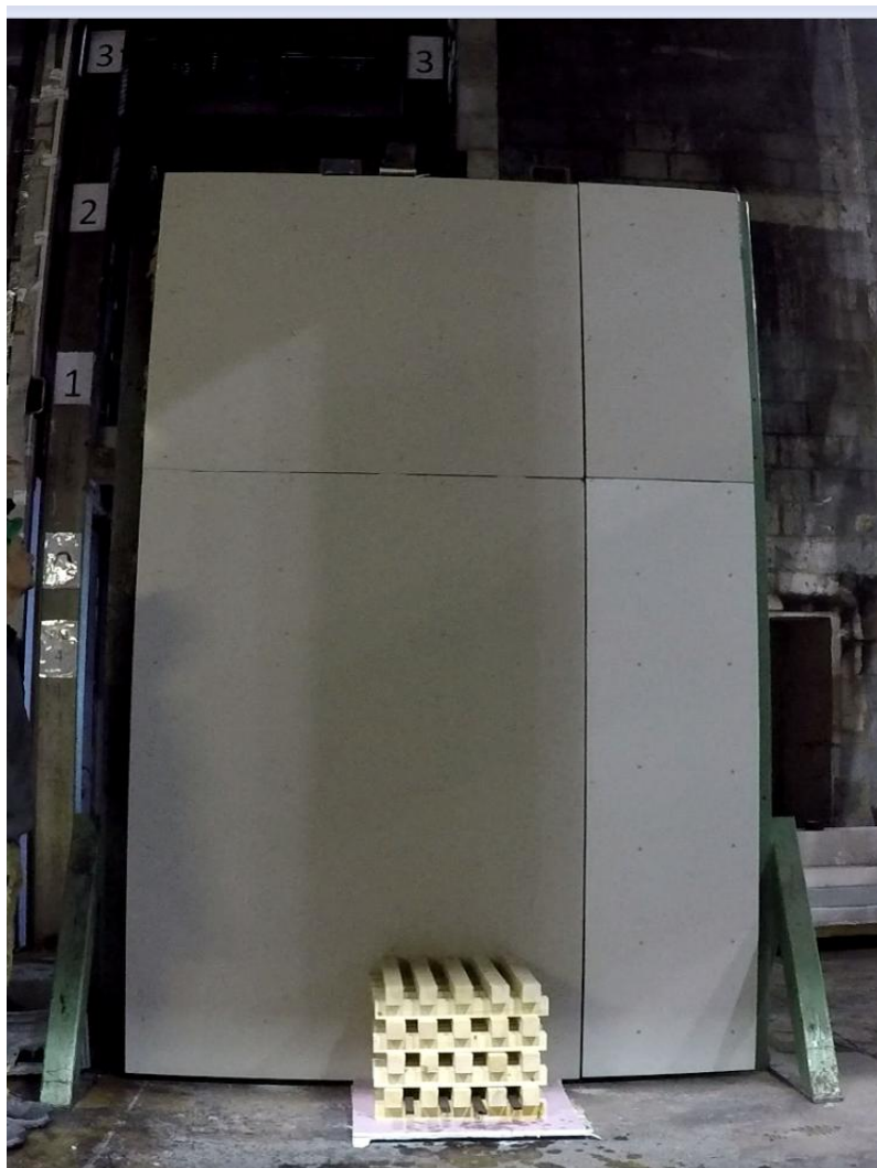
Figure D38 – ACM A2 panels installed on the experimental rig
