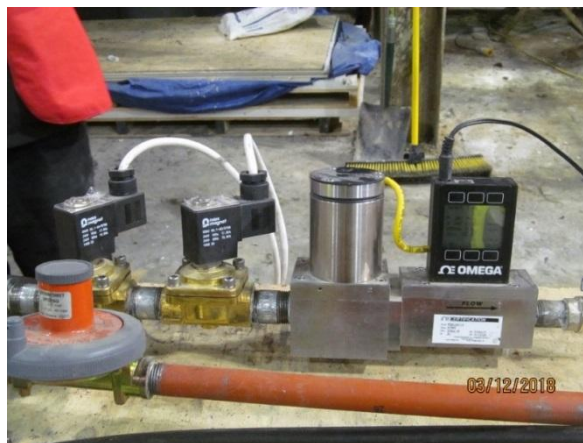
Figure D13 – Propane gas rig showing mass flow controller
