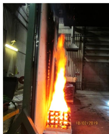
Figure D19 – Steady burning phase for Trial 1
