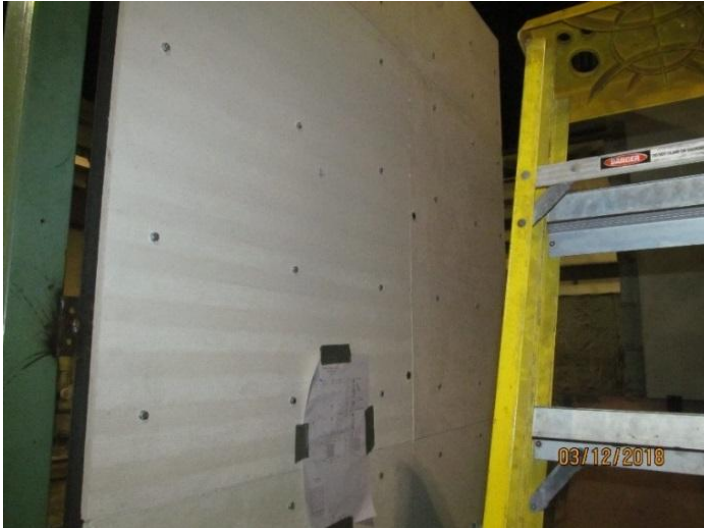
Figure D11 – Front face of experimental frame showing calcium silicate board
