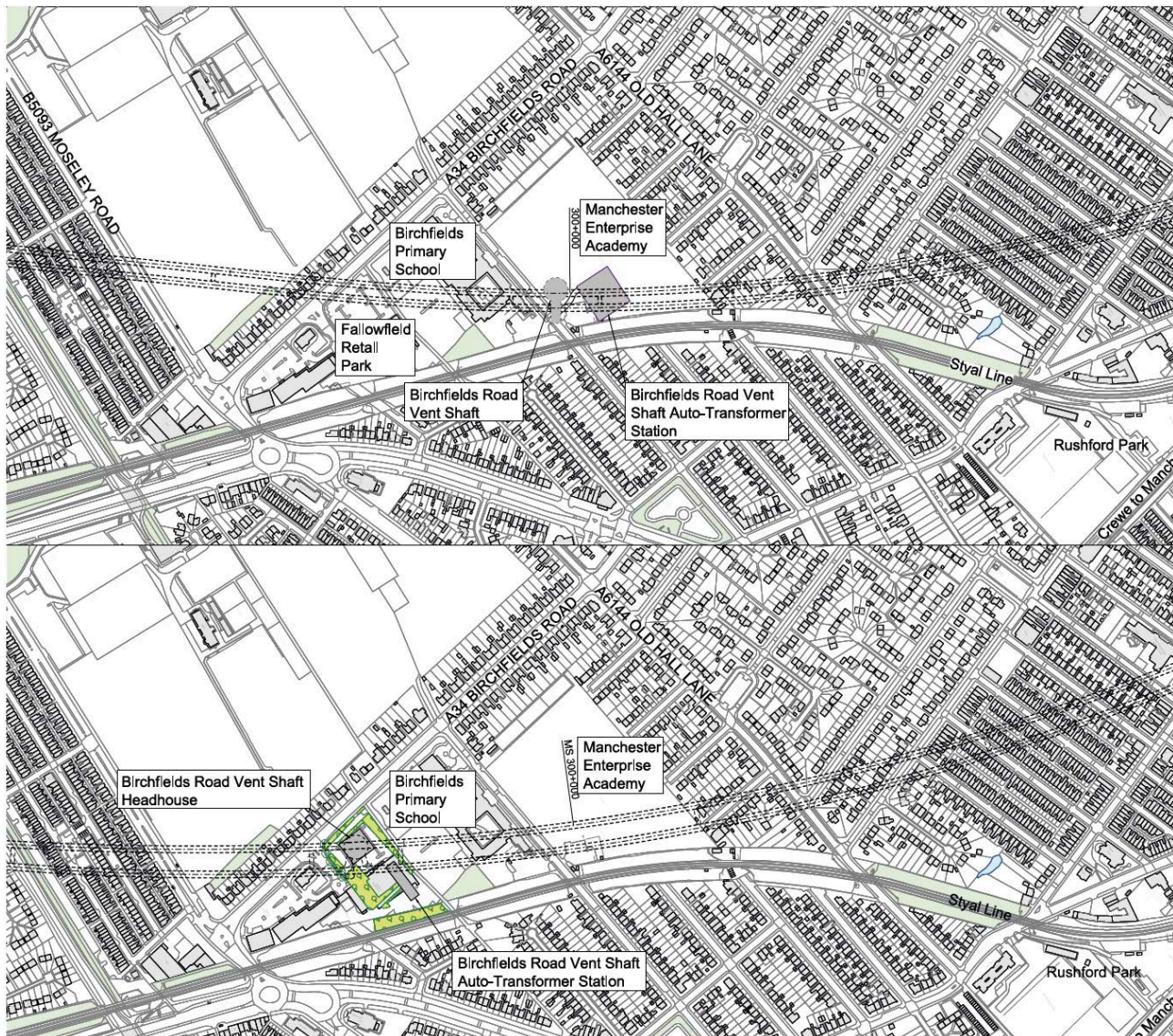
Figure 4: Plan showing the current design and proposed relocation of the vent shaft. For more detail see change two in Volume 2: Map book and visualisations.
