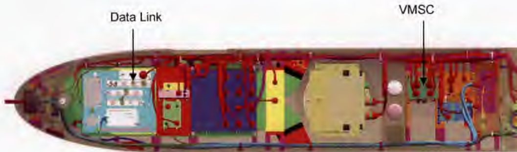
Figure 5 – Diagram of Front Compartment.
