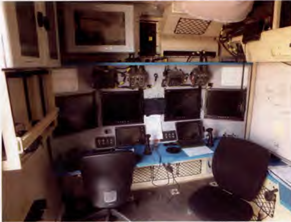
Figure 7 – Interior of GCS; note the computer screens are also known as Human Computer Interface (HCI).
