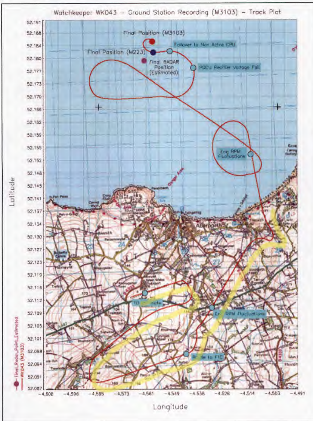
Figure 11 – VMSK flight data trace of WK043 from take-off to crash.
