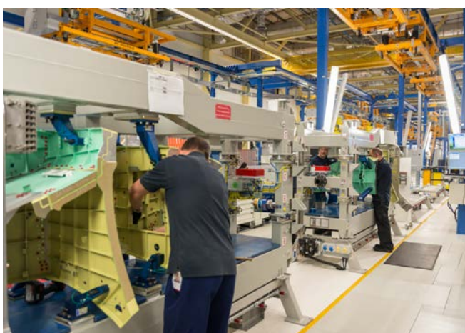
BAE Systems workers assembling the rear fuselage for the F-35 Lightning II, at their state of the art advanced manufacturing and assembly facilities in Lancashire, UK.
