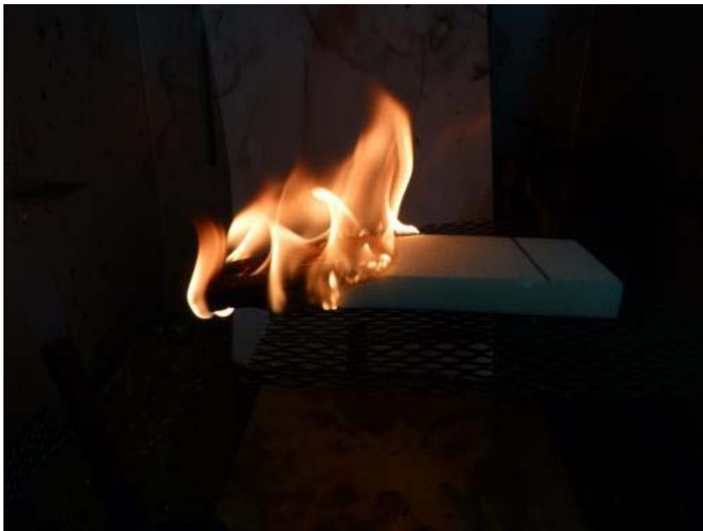
Photo 3 Foam insulation sample burning during tests (Courtesy: ITRI Innovation)
