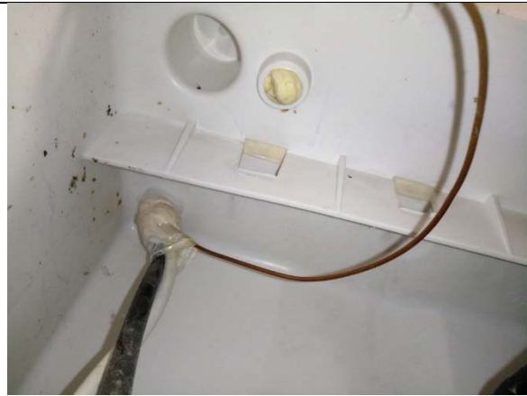
Photo 5 Compressor cavity, exposed foam fill point, cable and a capillary entry point.
