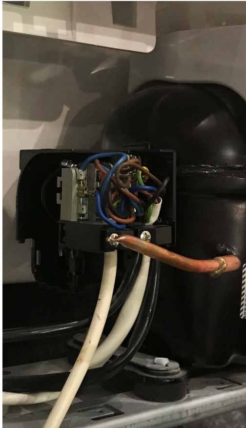
Figure 1: Mains cable attachment marking is on the removeable cover of the compressor
