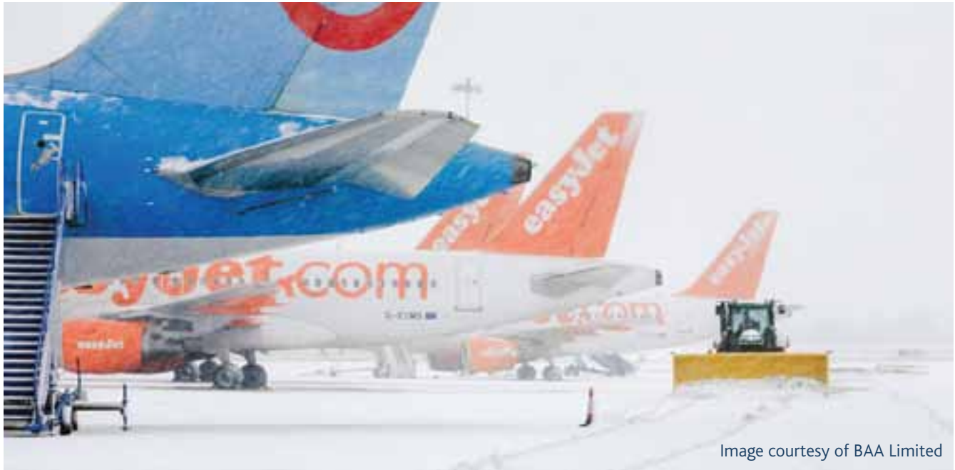
Figure 7.1 Clearing aircraft stands of heavy snow
