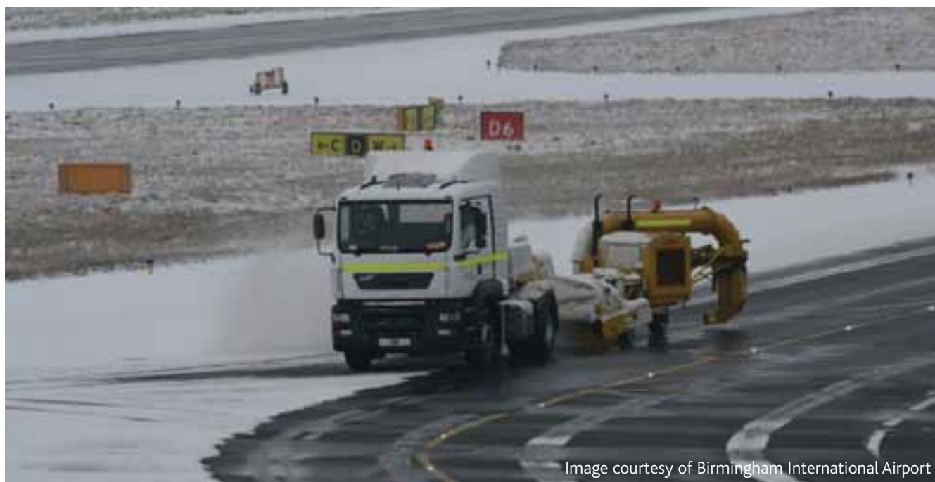
Figure 9.2 Clearing the taxiway at Birmingham International Airport
