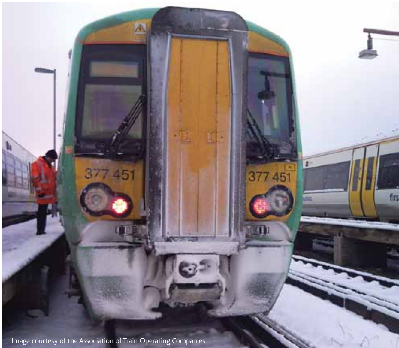
Figure 4.2 Snow impact on train automatic coupling and horn
