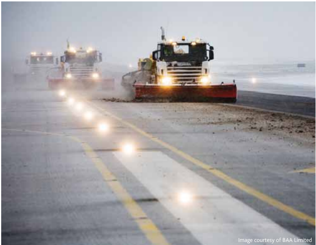
Figure 8.1 A fleet of snow ploughs clears a runway
